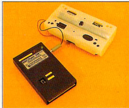
BBG is a battery backup RAM disk for GEOS 2.0 and GEOS 128.
