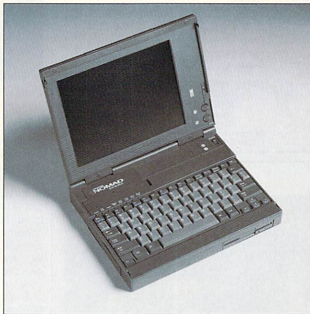
Gateway 2000's Nomad 450DXL notebook uses a new low-power version of the 486DX2/50 processor chip.
