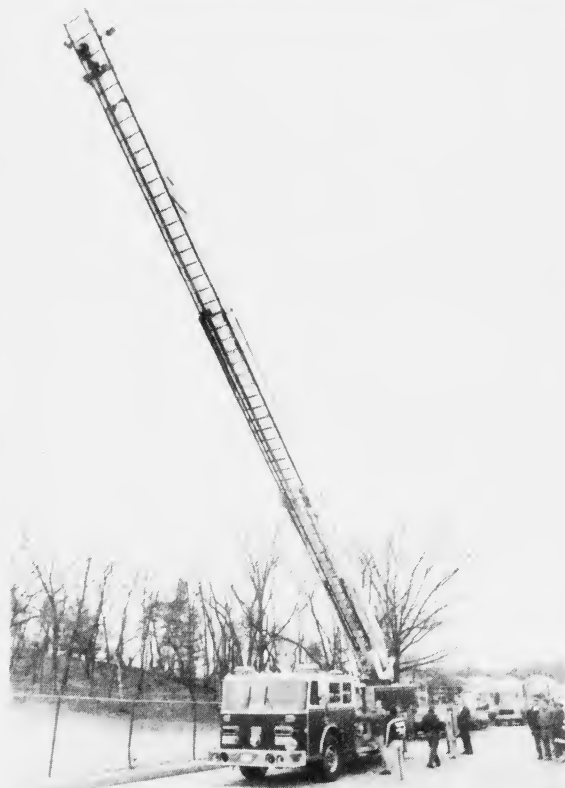
UP, UP, UP -- The 75-foot aerial ladder of the Quint Fire Truck is fully extended during a demonstration Monday for city officials and members of the Fire Department.
