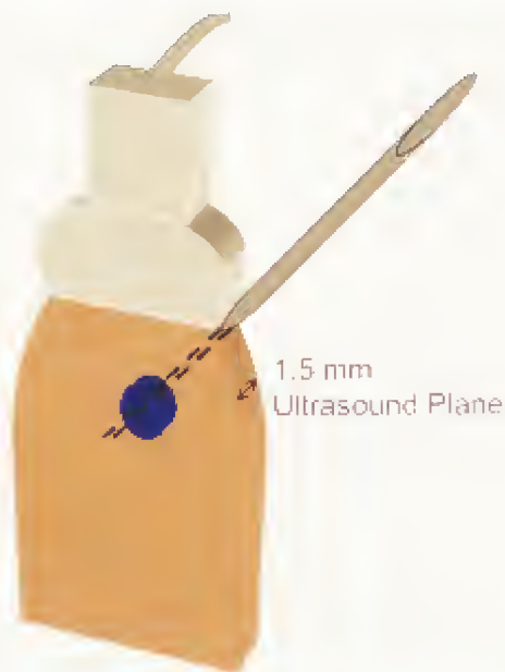
Figure 4–20. The ultrasound plane is approximately 1 to 1.5 mm thick. The biopsy needle must remain within this thin ultrasound plane at the same time that the lesion is maintained within that same plane to confirm accurate biopsy.
