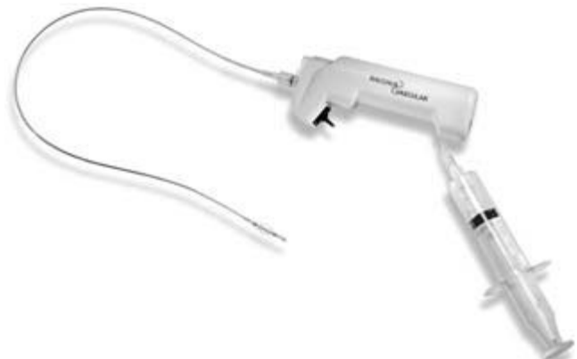
Figure 42.8 The Fino Thrombectomy Catheter (7 Fr). It is an over-the-wire catheter with an integral motor drive unit. It has a central hollow drive shaft connected to an expanding clot maceration and removal system.
