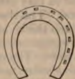
Fig. 1. Mr. Turner's Shoe (foot side), showing six nail holes on the outside, and two only on the inside, of the toe.
