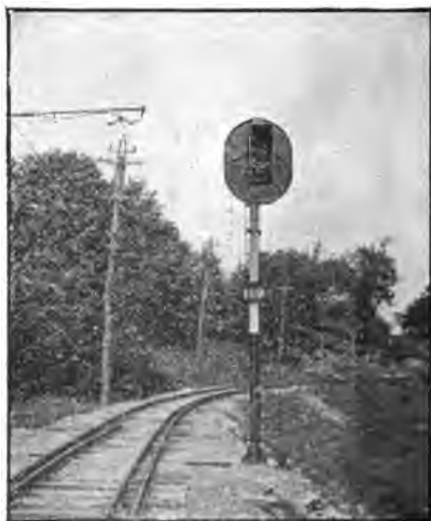
Fig. 203. Model 13 Light Signal Scranton and Binghamton Ry.
