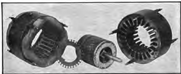
Fig. 145. Elements of the Induction Motor.
