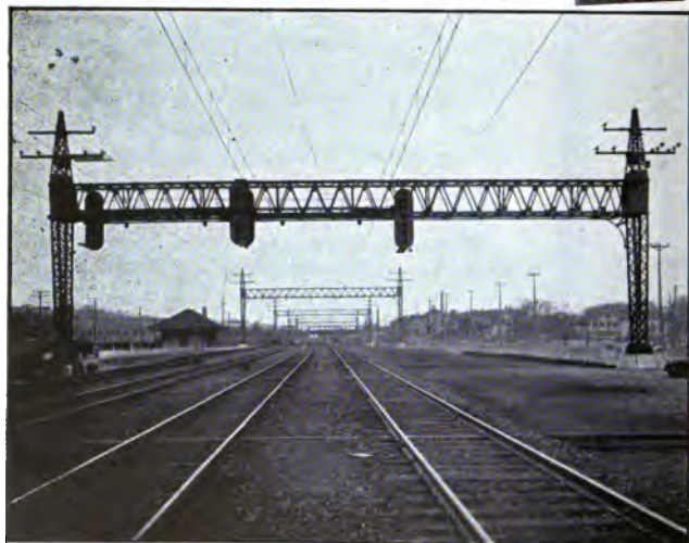
Fig. 171a. Model 14 Light Signals in Service on the New York, New Haven & Hartford R. R.
