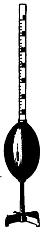
Fig. 75. — URINOMETER, made of metal, and with flanged foot (as supplied by Hicks, of Hatton Garden, E.C.).—The flanges steady it while in the urine, and form a stand when not in use.
