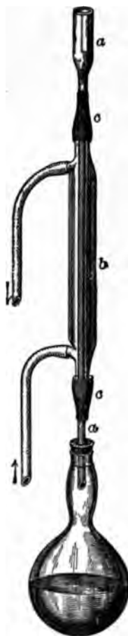
FIG. 9.—FLASK WITH REFLUX- CONDENSER.
