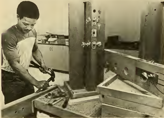
Apprentice Darryl Plummer mortises a door butt in Detroit's lock installation class.
