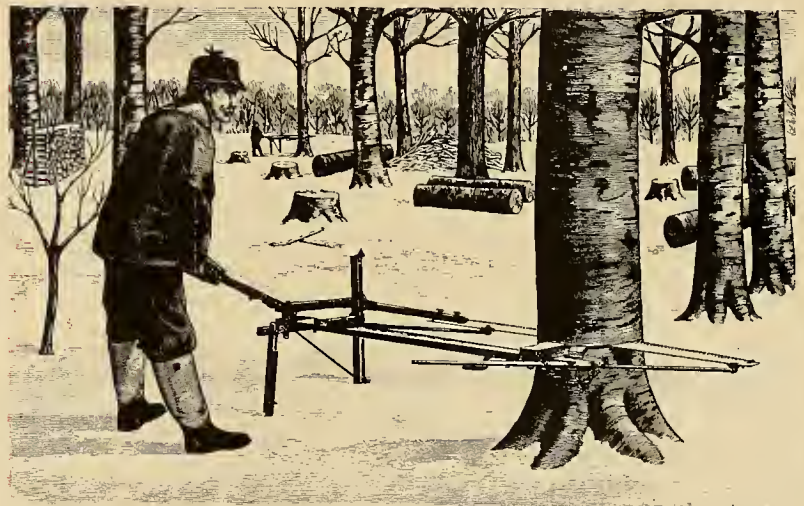
The folding saw machine could be set up as shown to saw down trees 18 inches and 27 inches from the ground, according to the 1890s catalog. It was hard work.
