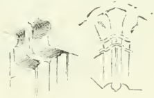
FIG. 225.—Glengarnock Castle. Caps at each side of a Fireplace.
