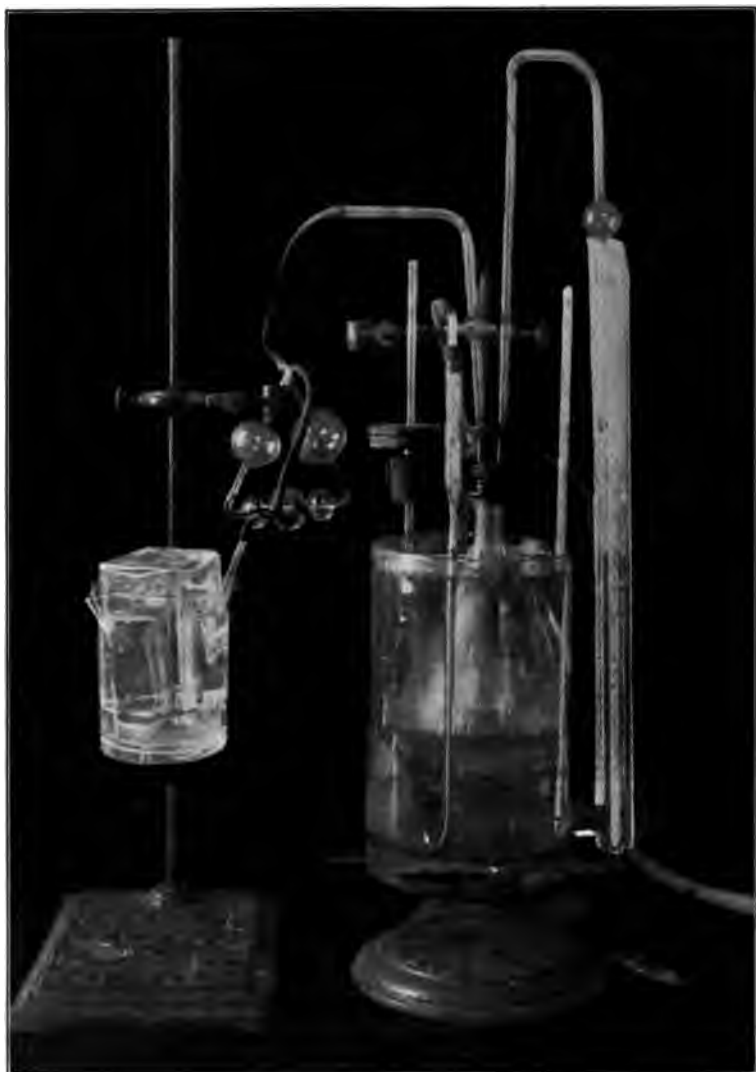
No. 46. DETERMINATION OF \text{CO}_2 AND \text{H}_2\text{O} IN DRYING OF LINSEED OIL — A piece of filter paper was immersed in pure linseed oil, and, after the absorbed oil was weighed, the filter paper was suspended in the Erlenmeyer flask, on the bottom of which was a solution of Barium Hydrate (free from \text{CO}_2 ) to absorb the \text{CO}_2 formed by the drying of the oil. The flask was immersed in a water-thermostat, the water of which was stirred by a revolving mechanical stirrer. A thermo-regulator, by means of which the gas-flame under the thermostat was automatically regulated, was placed under the flask. By opening the glass-cock, oxygen was admitted from time to time to the Erlenmeyer flask, and the absorption of oxygen was read on the mercury-manometer. The readings were always made at the same temperature. The oxygen, before entering the Erlenmeyer flask, was passed through the KOH bulb, where it was washed free from \text{CO}_2 . This experiment was conducted in triplicate with great care, the joints being all sealed with shellac and placed under mercury. No \text{CO}_2 or \text{H}_2\text{O} beyond a trace could be determined, owing to the small quantity of linseed oil which the filter paper contained.
