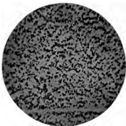
No. 23. AMERICAN WASHED OCHRE — Photomicrograph \times 250 , of the same composition as French ochre.
