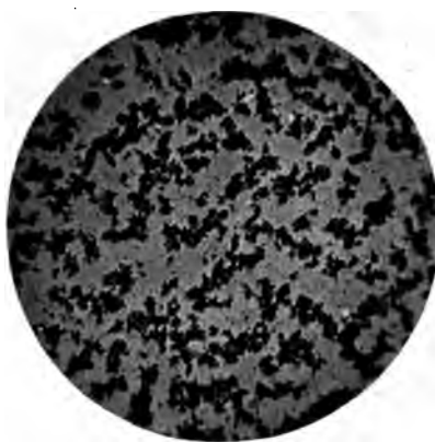
No. 22. ORDINARY AMERICAN WASHED OCHRE — Photomicrograph \times 250 , powdered and bolted; lower in iron than the French, but of uniform grain.
