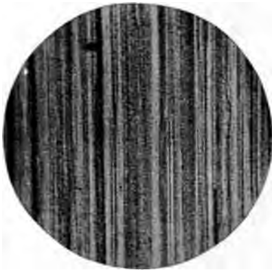
No. 26. ULTRAMARINE BLUE, ground in oil, very uniform and fine — Photomicrograph \times 250 .
