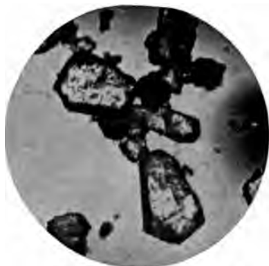
No. 66. TERRA ALBA (French Gypsum)— Photomicrograph \times 600 , showing crystalline structure of calcium sulphate.
