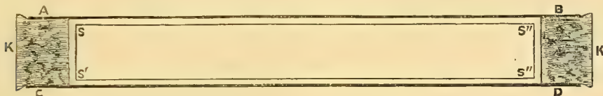
Fig. 31.—A, B, C, D, glass tube (can easily be cut to any length with a file); K K, corks closing ends; s, s', s'', sounding from tube.
