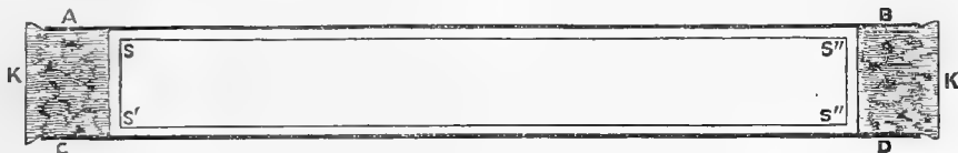
Fig. 51.—A, B, C, D, glass tube (can easily be cut to any length with a file); K K, corks closing ends; S, S', S'', soundings from tube.
