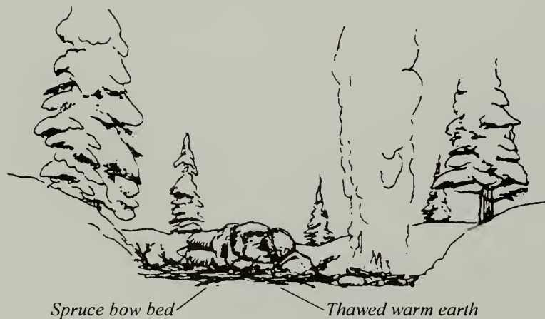
Heated earth camping place.
