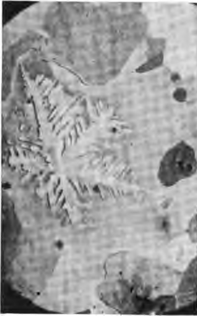
Fig. 9. (x 33 Diameters. Vertical Illumination.) Dendrites of Cadmium. Showing relation to crystallization.
