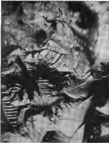
Fig. 11. (x 70 Diameters. Vertical Illumination.) Dendrites on Surface of Bismuth.
