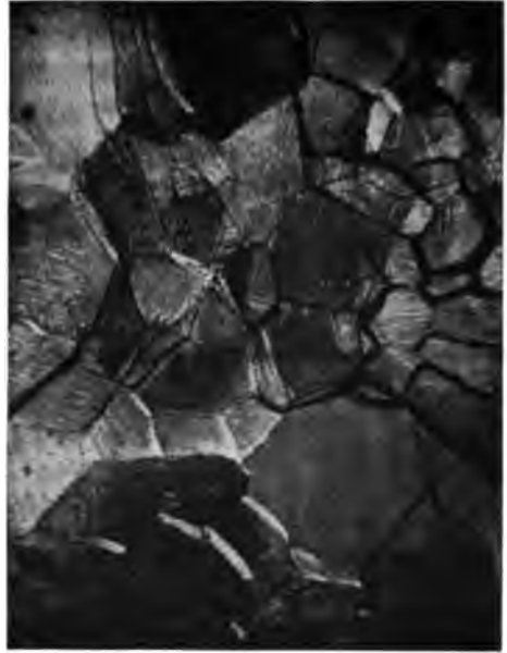
Fig. 6. (x 16 Diameters. Vertical Illumination.) Dendrites on Surface of Silver. Showing relation to crystallization.
