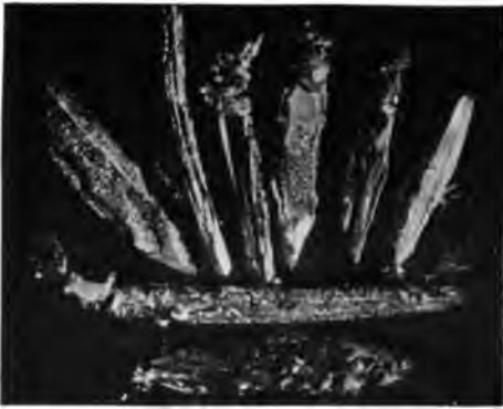
Fig. 25. (x 15 Diameters. Oblique Illumination.) Crystals of Electrolytic Silver.
