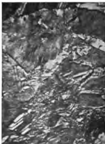
Fig. 24. (x 33 Diameters. Oblique Illumination.) Section of Knob from Electrolytic Copper.
