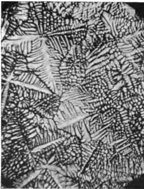
Fig. 3. (x 35 Diameters. Vertical Illumination.) Dendrites on Surface of Aluminum.
