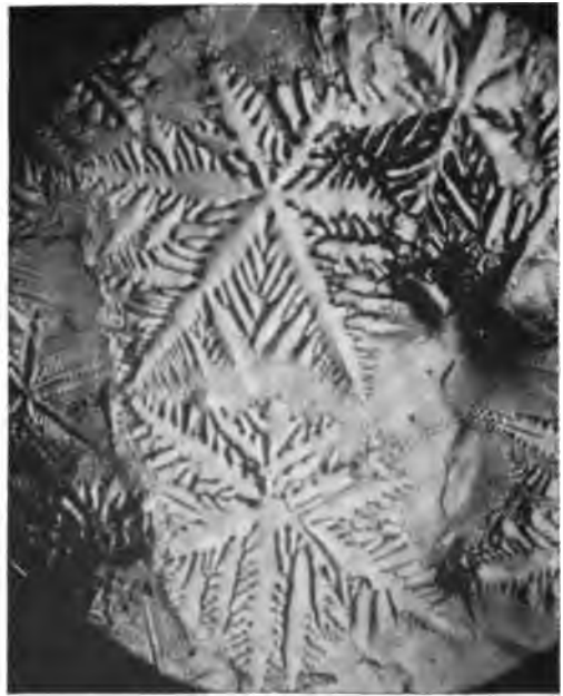
Fig. 8. (x 33 Diameters. Vertical Illumination.) Dendrites on Surface of Cadmium. (Same Ingot as Fig. 7.)
