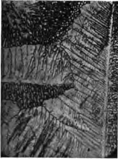
Fig. 13. (x 30 Diameters. Vertical Illumination.) Dendritic Structure of Tin Cast on Stone.
