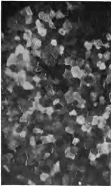
Fig. 7. (x 30 Diameters. Oblique Illumination.) Cadmium Cast in Iron Mold and Etched with Nitric Acid.
