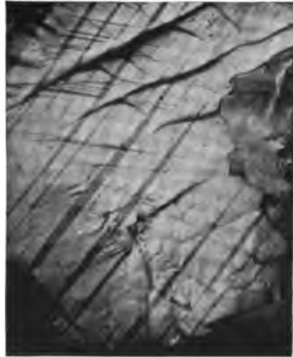
Fig. 12. (x 33 Diameters. Vertical Illumination.) Slip Lines on Strained Bismuth.
