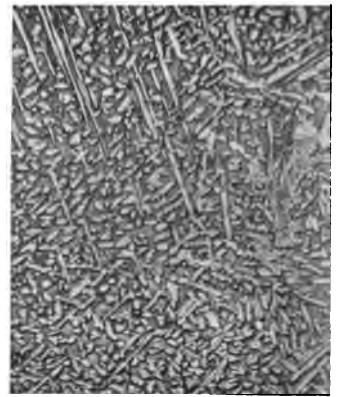
Fig. 33. (x 35 Diameters. Vertical Illumination.) Polished Section near base of Cu-Al Alloy. Shows dendrites.
