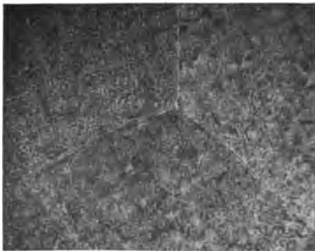
Fig. 29. (x 35 Diameters. Vertical Illumination.) Polished Section near top of Cu-Al Alloy, after being heated, quenched, reheated, and slowly cooled.
