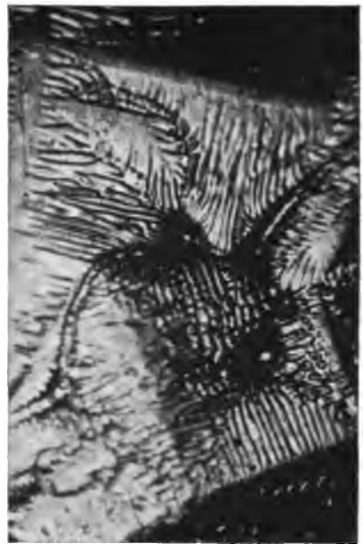
Fig. 4. (x 33 Diameters. Vertical Illumination.) Dendrites on Surface of Platinum.
