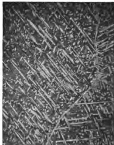
Fig. 35. (x 35 Diameters. Vertical Illumination.) Polished Section near base of Cu-Al Alloy, corresponding to Figs. 33 and 34.
