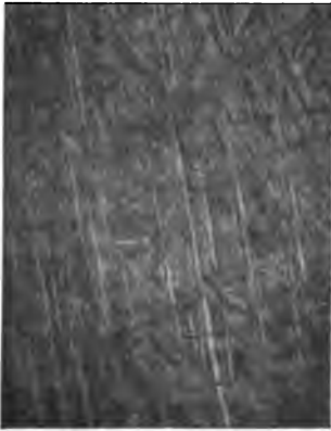
Fig. 31. (x 35 Diameters. Vertical Illumination.) Polished Section near center of Cu-Al Alloy. Shows new structure.
