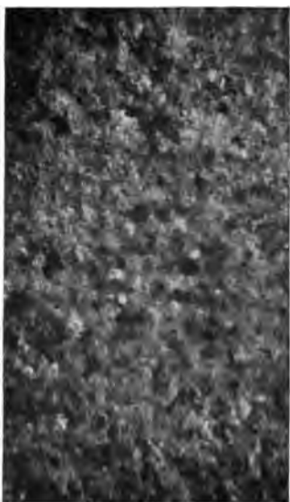
Fig. 17. Structure of Cast Tin Hammered to a Thickness of 0.02 in.
