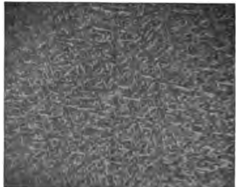
Fig. 30. (x 200 Diameters. Vertical Illumination.) Polished section near center of Cu-Al Alloy.
