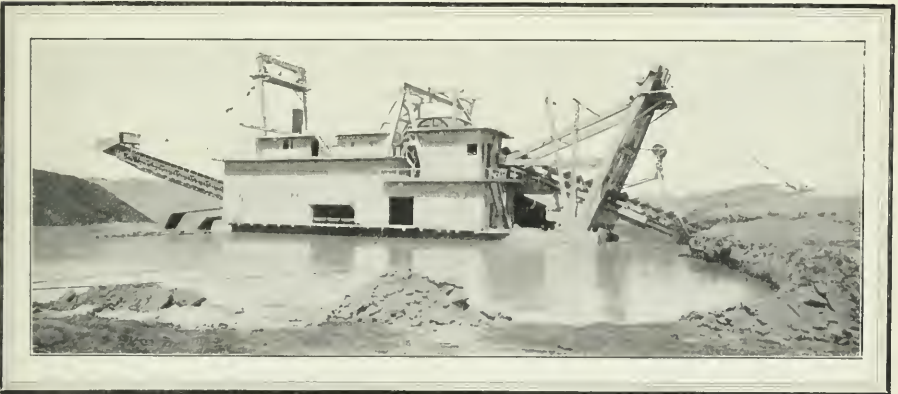
A typical gold dredger at work; the digging end at the right
