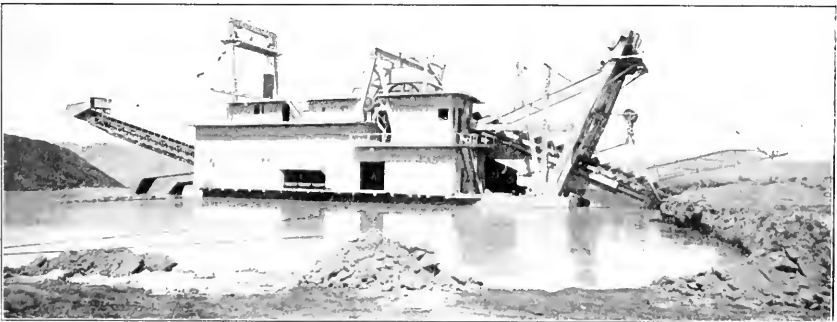
A typical gold dredger at work; the digging end at the right
