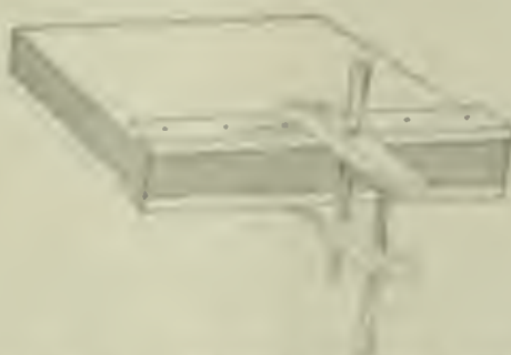
FIG. 1. VOLUME CLAMPED FOR DRILLING HOLES
