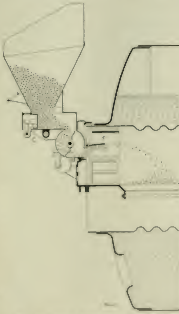
FIG. 2. LEACH STOKER AS MADE AT MÜHLBERG, GERMANY
