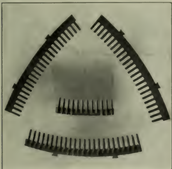
FIG. 5. CORE LAMINATIONS, A FINGER PLATE AND A VENTILATING SPACER
