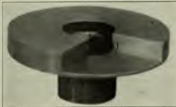
FIG. 3. FLANGE SHOWING FINISHED JOINT
