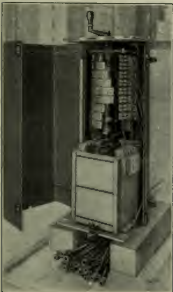
FIG. 4. SPEED CONTROLLER WITH CAM-OPERATED STATOR SWITCH
