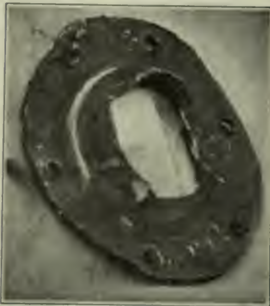
TWO VIEWS OF LEAD GASKET
