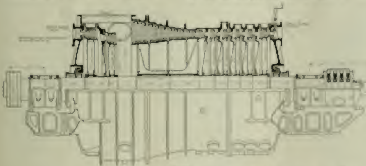
FIG. 2. 7,500-HORSEPOWER CURTIS TURBINE FOR SCOUT CRUISER
