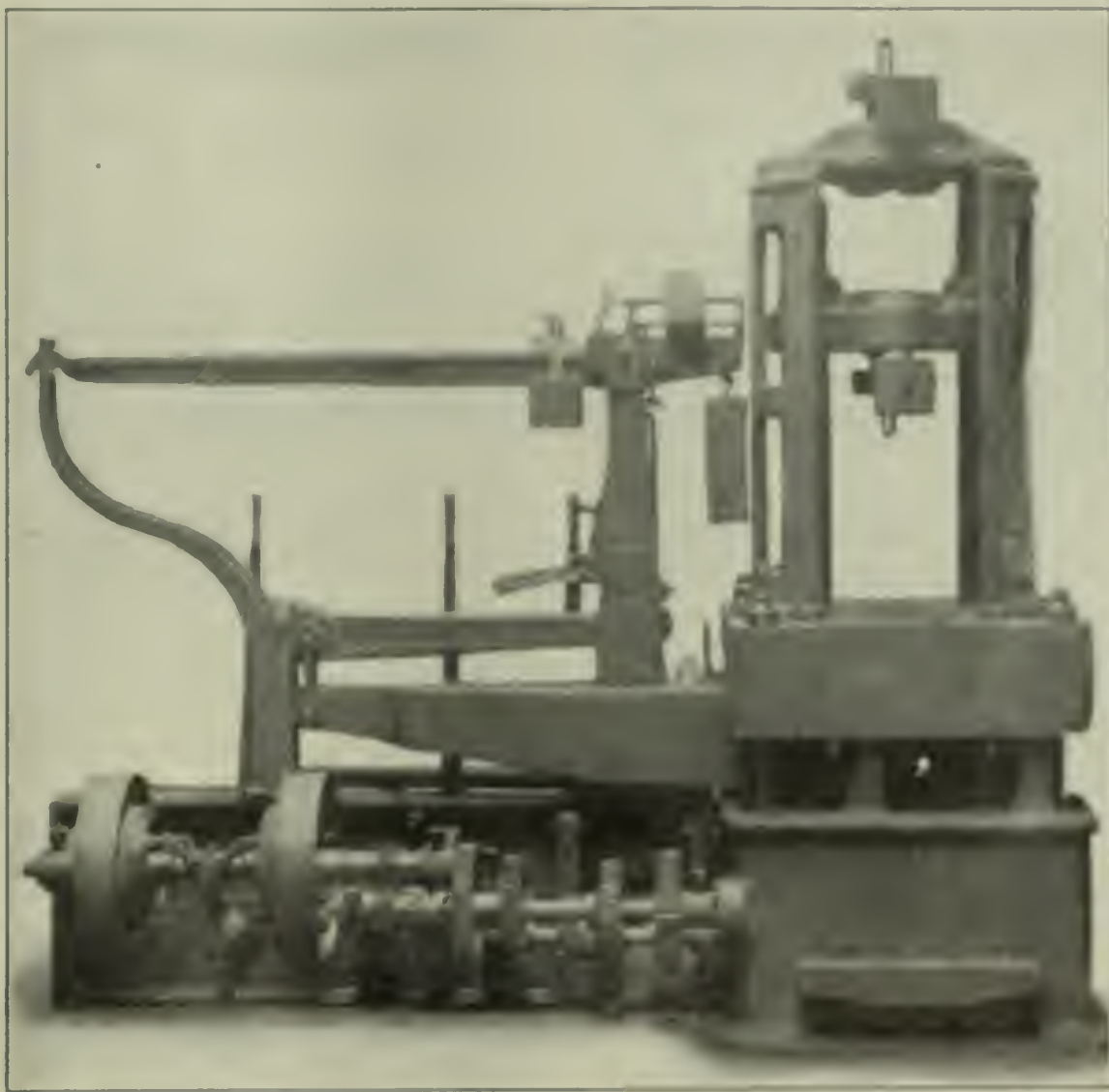
FIG. 1. TESTING MACHINE SHOWING DRIVING GEARS
