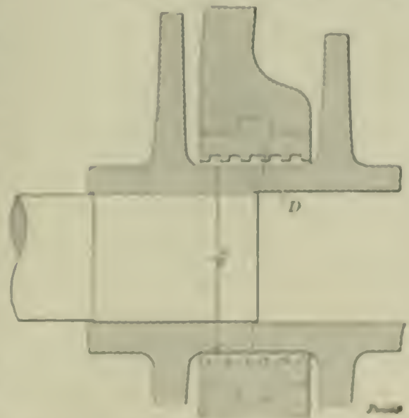
FIG. 11. STUFFING BOX OF A RATEAU STAGE.
