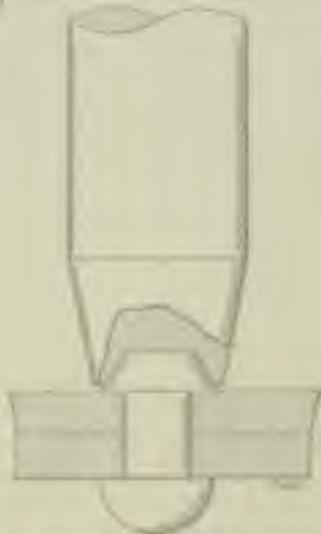
FIG. 2. CORRECT METHOD OF FORMING RIVET HEAD
