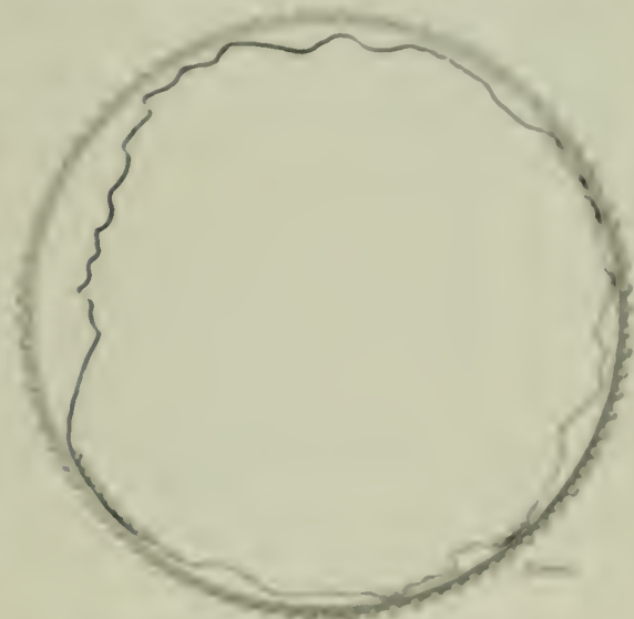
RUPTURED HEAD OF AIR TANK
