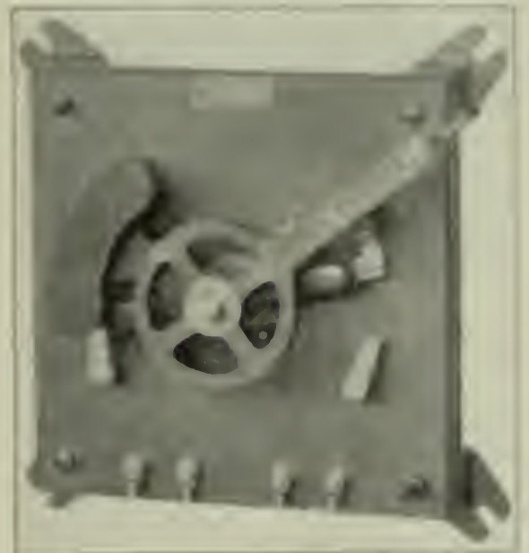
FIG. 6. FLOAT SWITCH WITH OPERATION BY ROPE.
