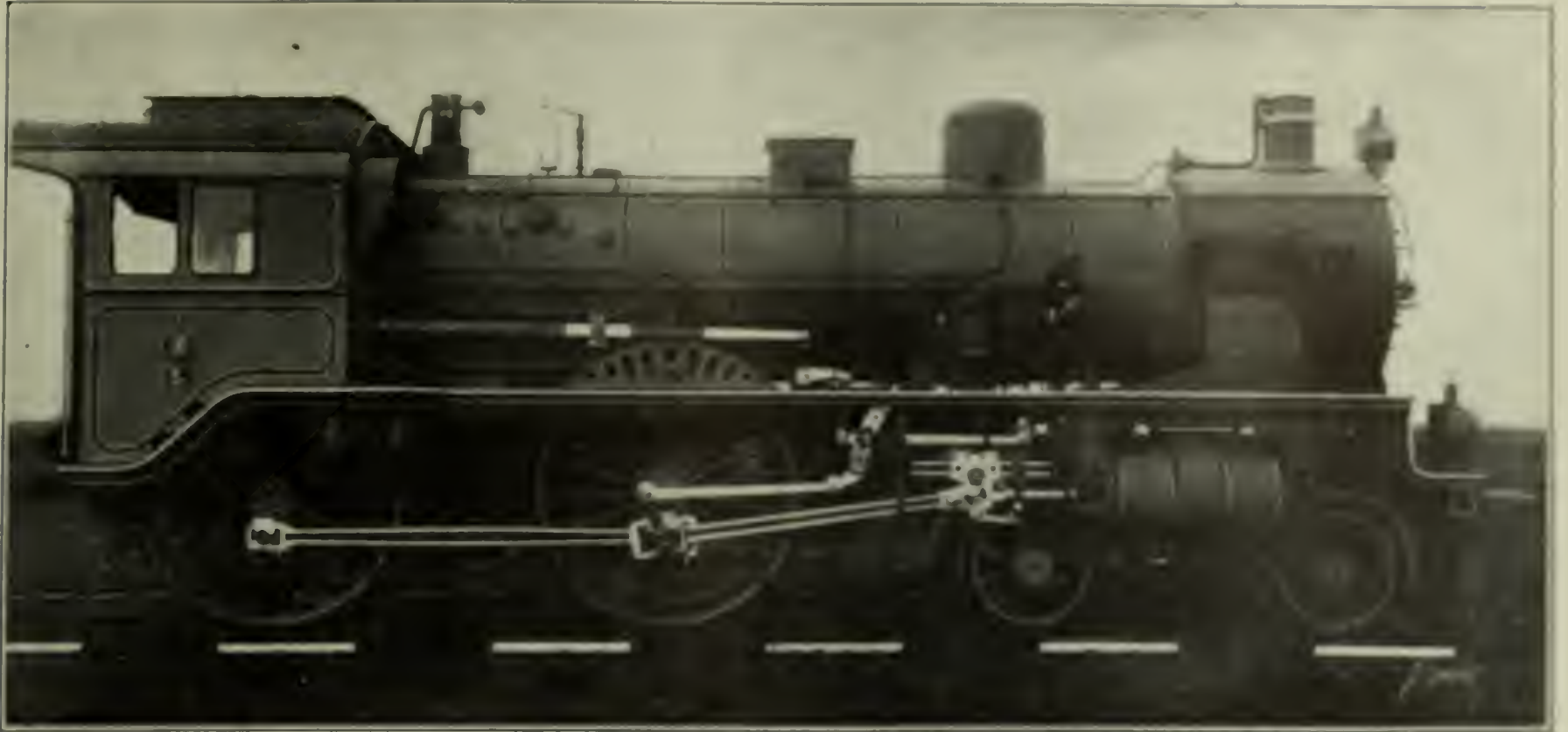
FIG. 2. AN EXPRESS LOCOMOTIVE UTILIZING STUMPF PATENT
