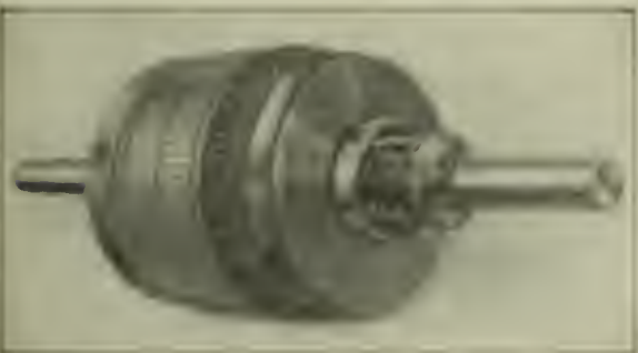
FIG. 367. ROTOR OF CUMMANS-SPEED SINGLE-PHASE MOTOR SHOWN IN FIG. 365. COMMUTATOR END
