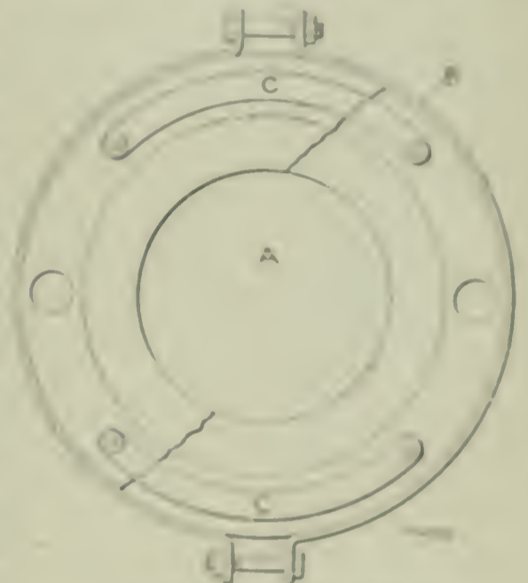
REPAIRED PUMP GLAND
