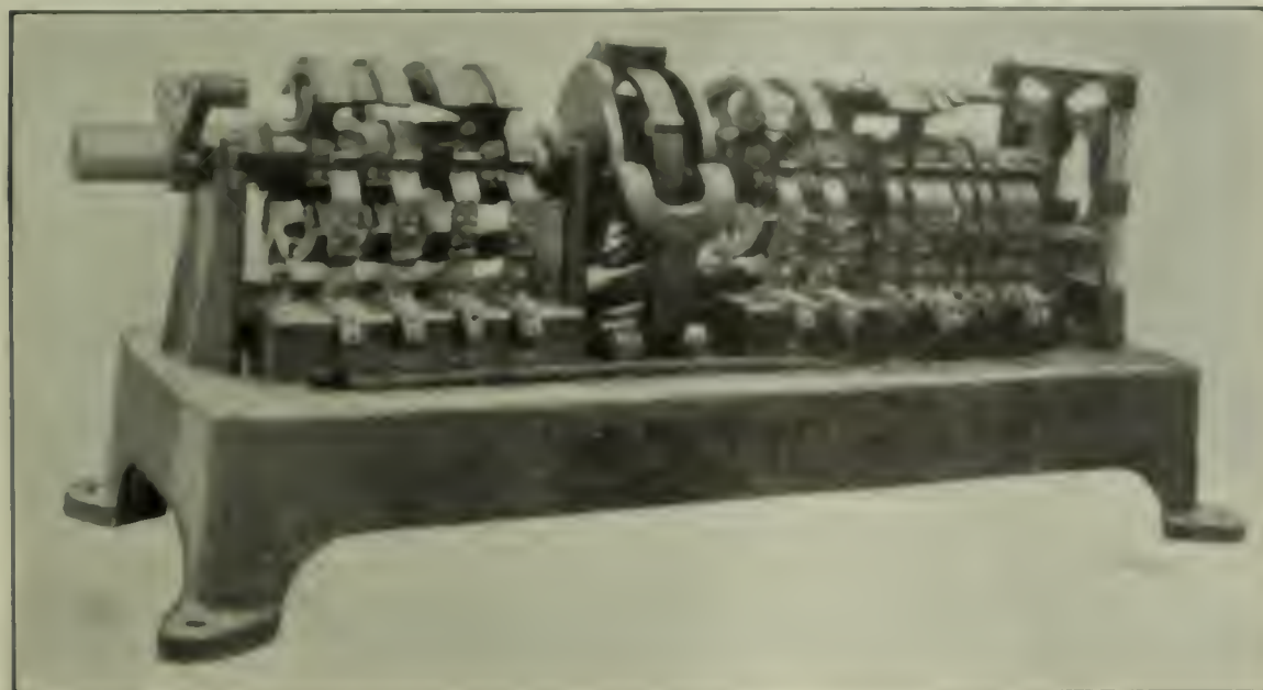
FIG. 10. HORIZONTAL CONTROLLER FOR ELEVATOR SERVICE
