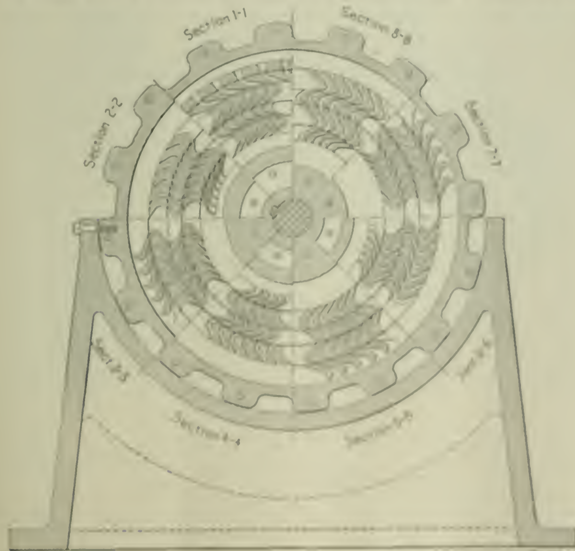
FIG. 2. PARTIAL CIRCUMFERENTIAL THROUGH LINES 1-1 TO 8-8
