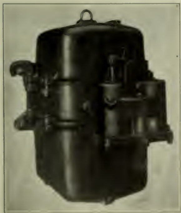
FIG. 10. SMALL STARTER ACTUATED BY PRESSURE RELAY
