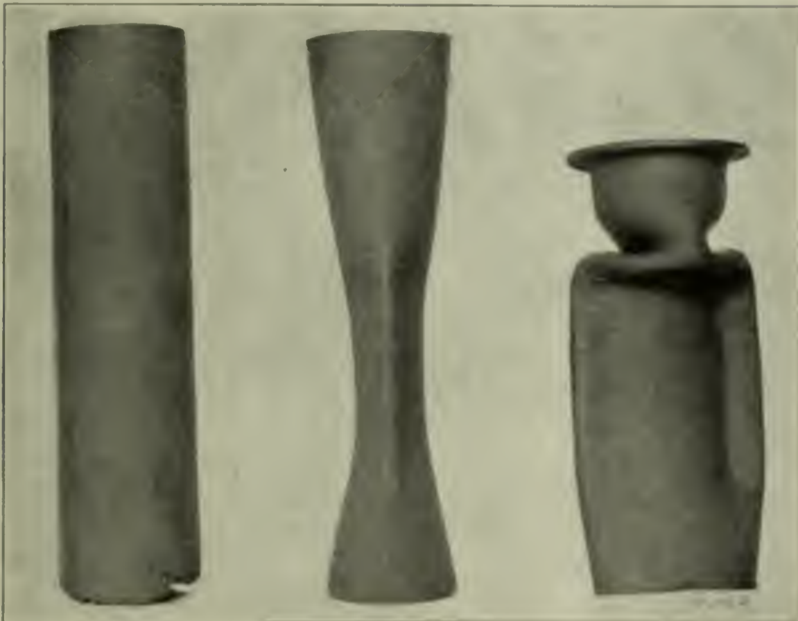
TUBE SUBJECTED TO CRUSHING-DOWN AND FLATTENING TESTS
