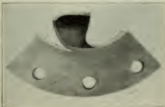
FIG. 1. METAL STRIPPED BY DRIFTING TOOL, SHOWING NO FUSION
