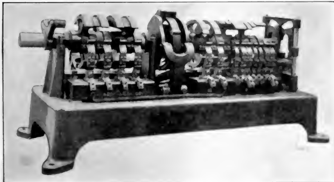
FIG. 10. HORIZONTAL CONTROLLER FOR ELEVATOR SERVICE
