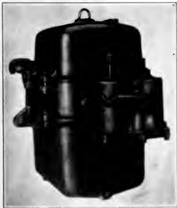
FIG. 10. SMALL STARTER ACTUATED BY PRESSURE RELAY
