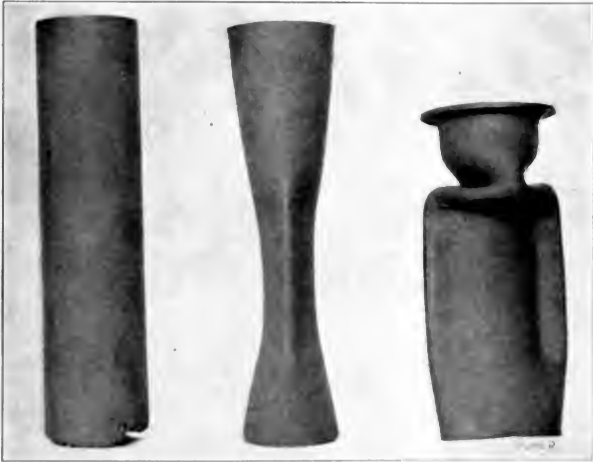
TUBE SUBJECTED TO CRUSHING-DOWN AND FLATTENING TESTS
