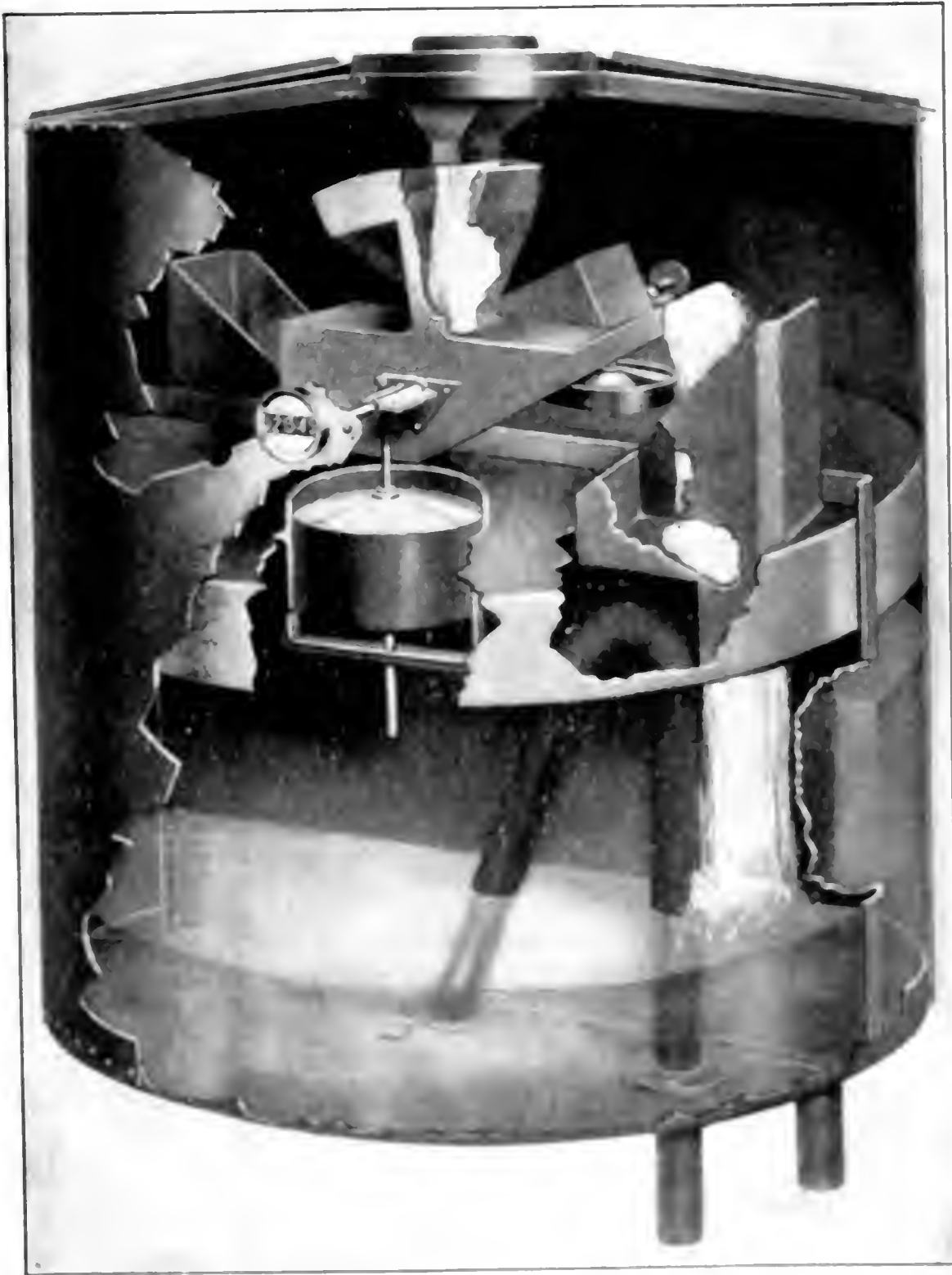
FIG. 1. VIEW SHOWING INTERIOR OF THE KENNICOTT WATER WEIGHER.
