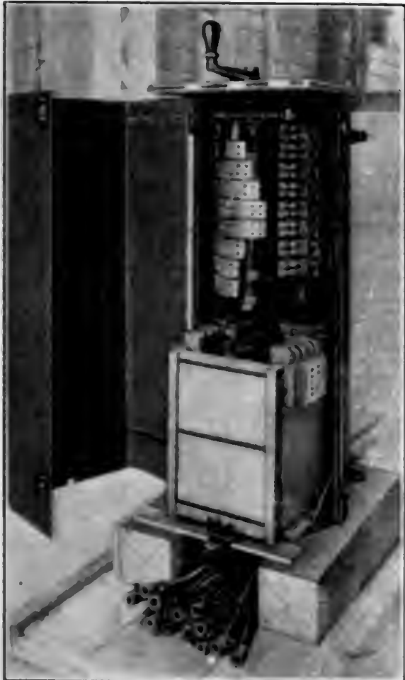
FIG. 4. SPEED CONTROLLER WITH CAM-OPERATED STATOR SWITCH
