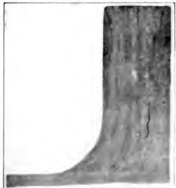
FIG. 2. METAL STRIPPED BY DRIFTING TOOL, SHOWING FUSION
