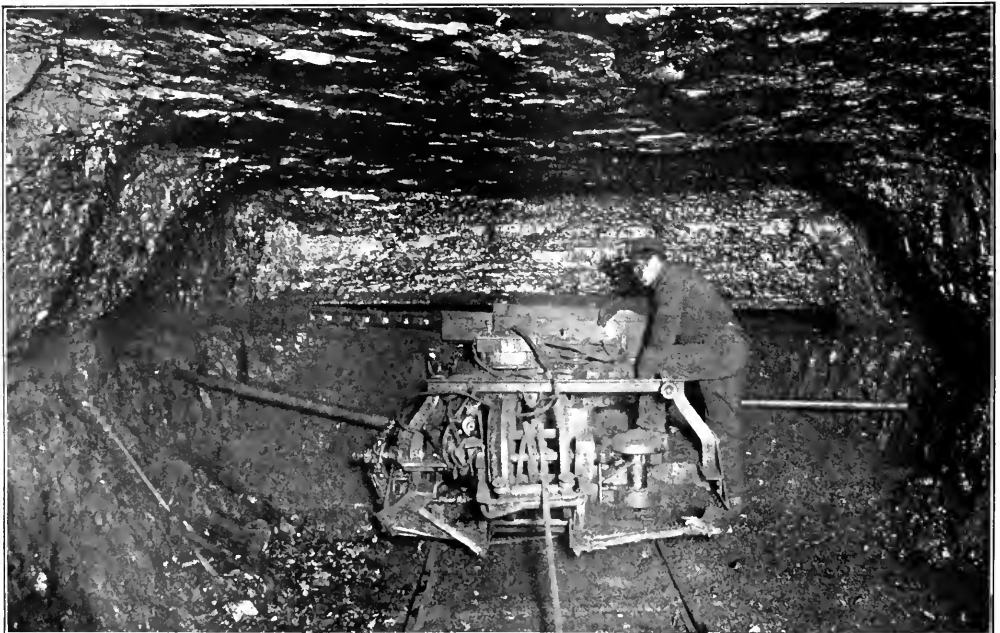
FIG. 1. CUTTING MACHINE REMOVING THE BONE BINDER FROM BETWEEN THE TWO SEAMS OF COAL
