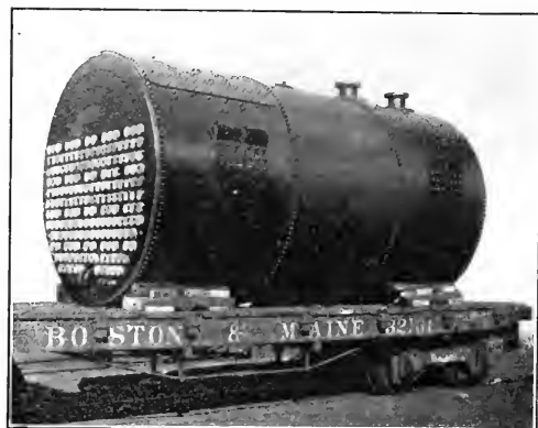
NINE-FOOT RETURN-TUBULAR BOILER READY FOR SHIPMENT
