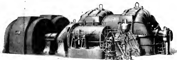
A 40,200-hp. PARSONS-TYPE TURBO-GENERATOR of 1915
