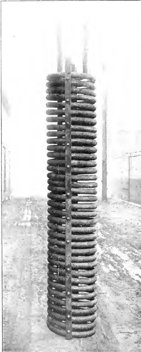
FIG. 8. PIPE COIL FOR AMMONIA PLANT; HAS 180 FT. OF PIPE.
