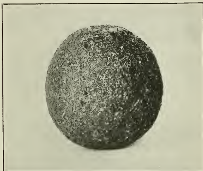
FIG. 3. BALL OF PUTTY AFTER BEING IN TEST FURNACE
