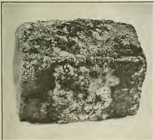
FIG. 2. BRICK THAT HAS BEEN PAINTED AND EXPOSED TO HIGH TEMPERATURE
