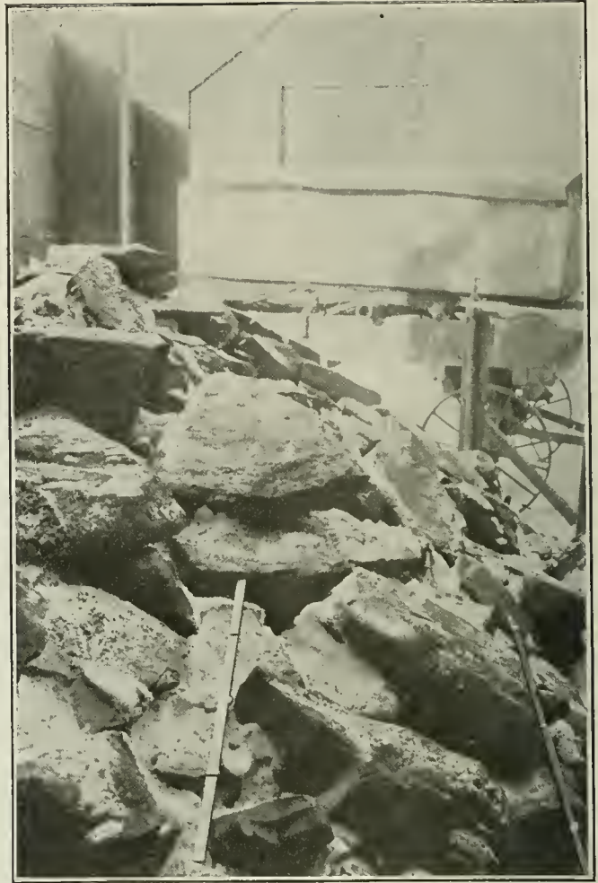
FIG. 1. SLATE AND STONE TAKEN FROM COAL SOLD IN NEW ENGLAND. NOTE THE TWO-FOOT RULE
