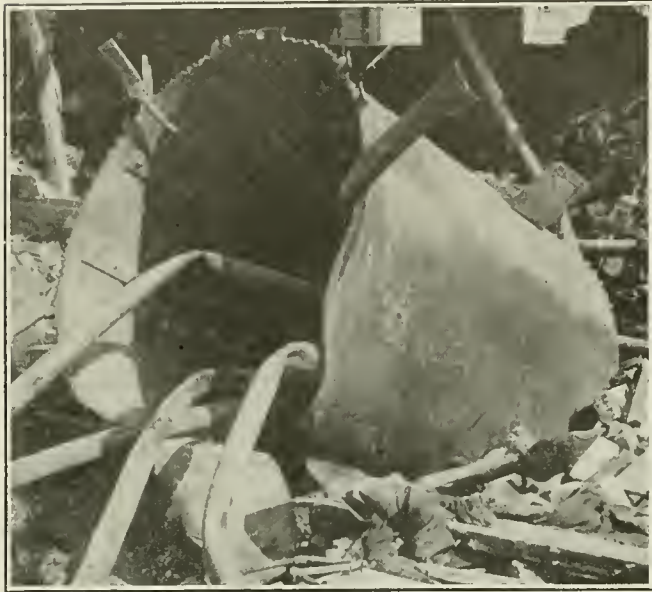
FIG. 2. REAR SHEET OF THE EXPLODED BOILER
