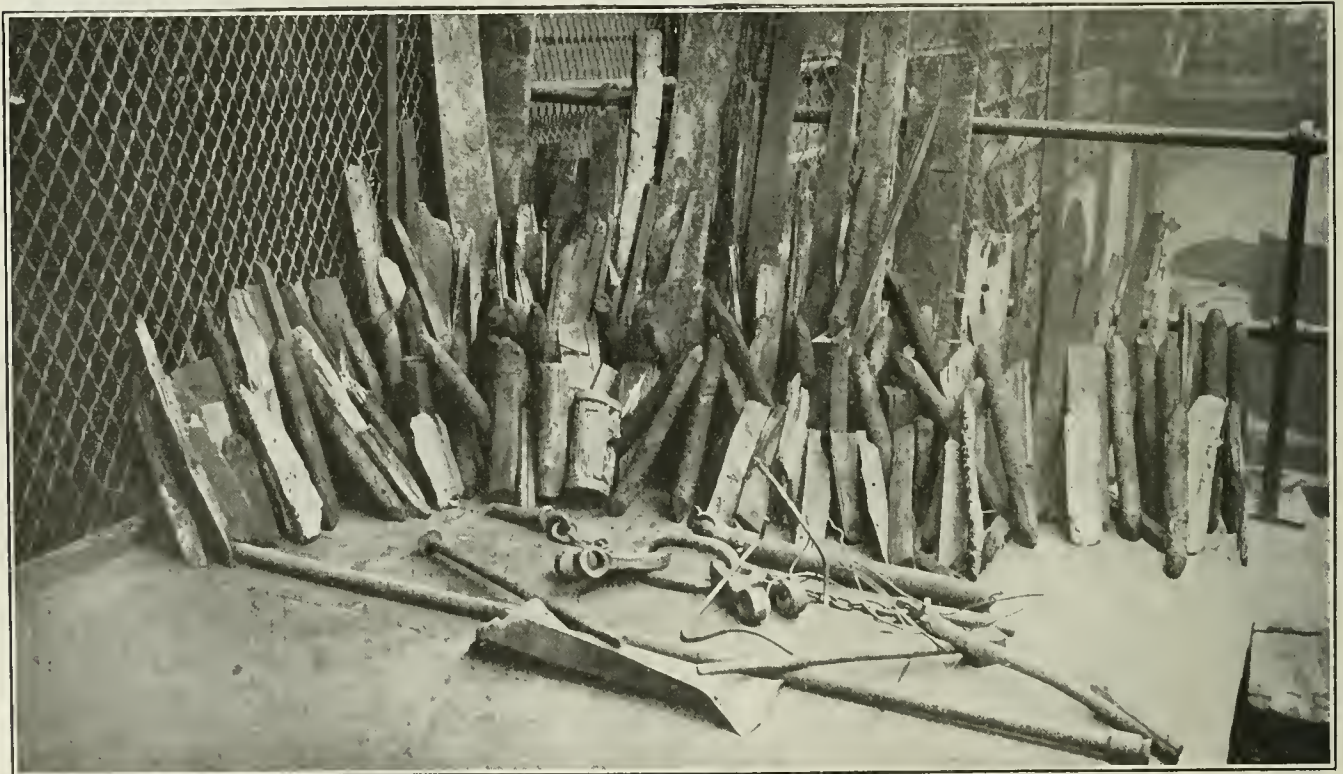
FIG. 2. SOME THINGS THAT COME IN COAL AND DAMAGE THE CRUSHER AND STOKERS
