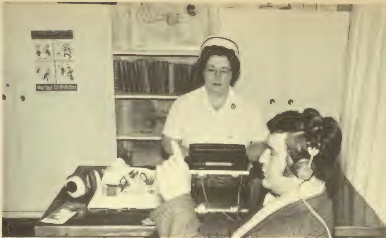
Those who work in high-noise areas of the plant have an audiogram every eight months to a year. Miss Hamilton, who has special training in audiometry, tests the hearing of one of the company's employees.
