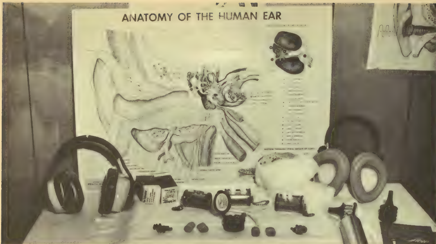
An assortment of hearing protectors worn by employees in high noise areas. In some industries, where extremely high noise levels prevail, a helmet-type protector (not shown) is used by the employees.
