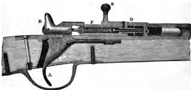
FIG. 21.—THE CHASSEPOT RIFLE.—SECTION OF THE BREECH.
